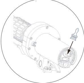
Clean the air inlet at the back of the hot air blower.
