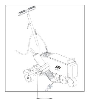
Use steel brush to clean the welding nozzle.
