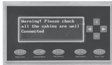
Pic6 Frequency Lockout Warning
