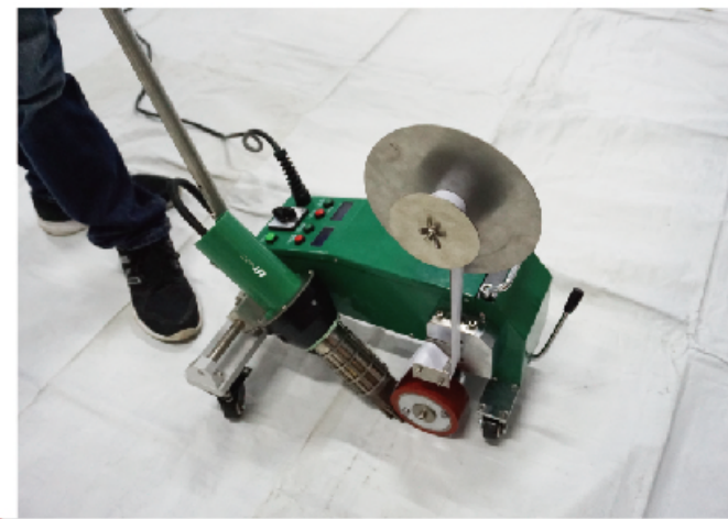
Tape Welding of Tarpaulin LST-MAT2
