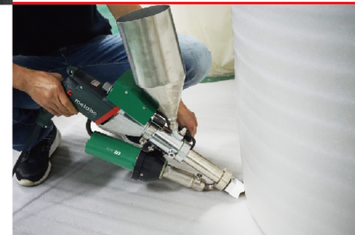
Plastic Tank Welding LST620
