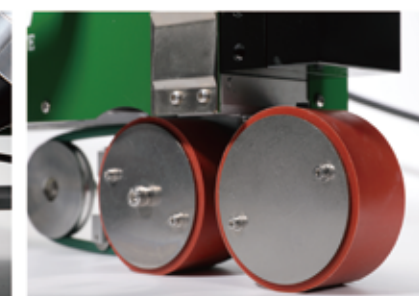
Advanced Belt Combined with Pressure Rollers System
